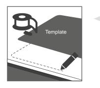
Select the installation place for the sink. Make sure that the surface is completely level and there is enough space under the countertop to fasten the brackets. Place the template on the countertop at the selected place, fix it with scotch tape and check whether it is in correct position. Outline the template with a marker.
